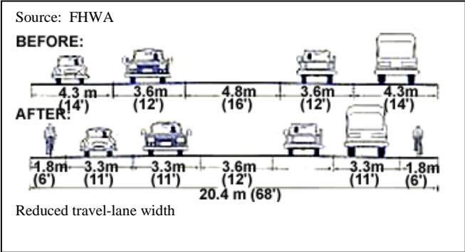
Road restriping example - an existing five lane road with 12’ lanes (total 60’ of road width) could be adjusted to five 10’ lanes and 5’ bike lanes (total 60’ of road width).
